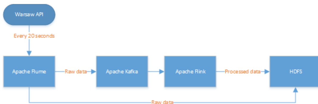
Figure 4: Trams and buses locations data flow
